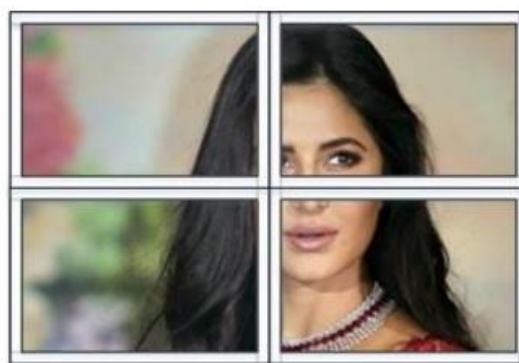
Correct Bezel Compensation
