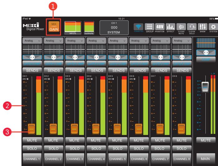
1. MIX / GAIN function switch: A switch that switches the fader to control channel level or control channel gain.
